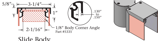
Slide Body Part #1260 For Removable Faces
